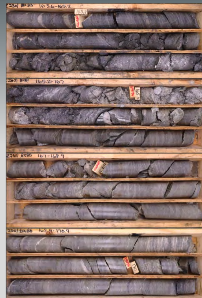
Drill core from drillhole SZ2301 (3.5 metres at 1.93 g/t Au and 57.5 g/t Ag starting at 163.8m)
