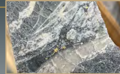
Native 'free gold' in drill core from hole GS2335 (3.1-metres at 39.5 g/t Au from 142.3m)
