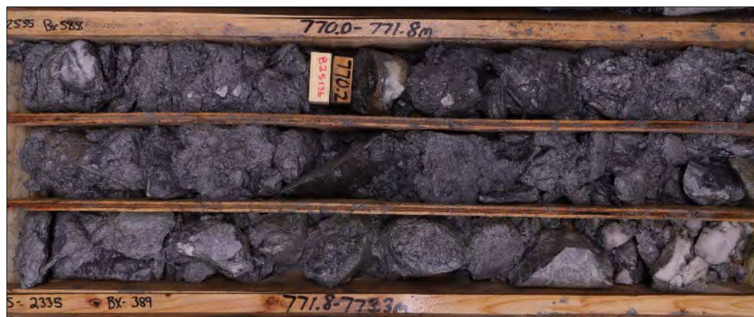
Figure 7-12 DDH GS2335, Newsboy Sinistral Fault Breccia, Gouge Zone
