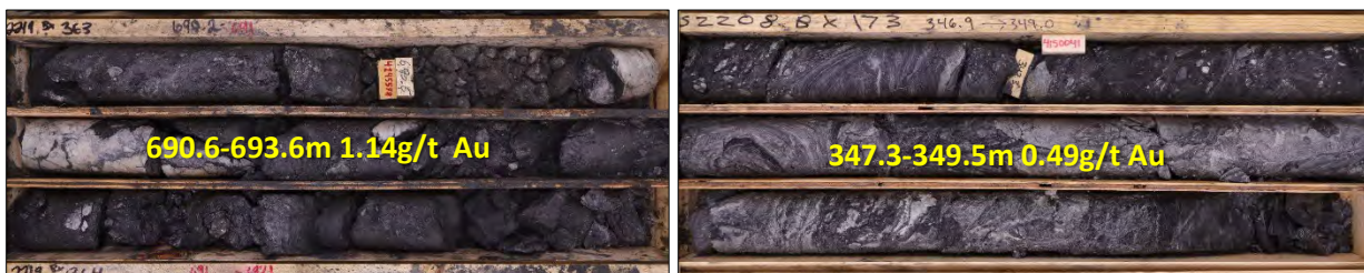
Figure 7-18 DDH GC2208 (left) and GS2219 (right) intersected respectively Cleary Road Cut and Tolovana Shears
