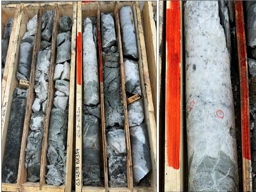
Figure 7-22 Drill hole GS2518 Altered Schists, with Massive Quartz Veining, Visible Gold
