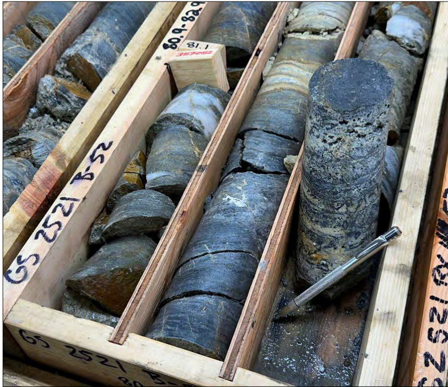
Figure 7-21 Drill hole GS2521, 82 m, Base Metal Mineralization, Signature of Upper Level Gold Mineralization
