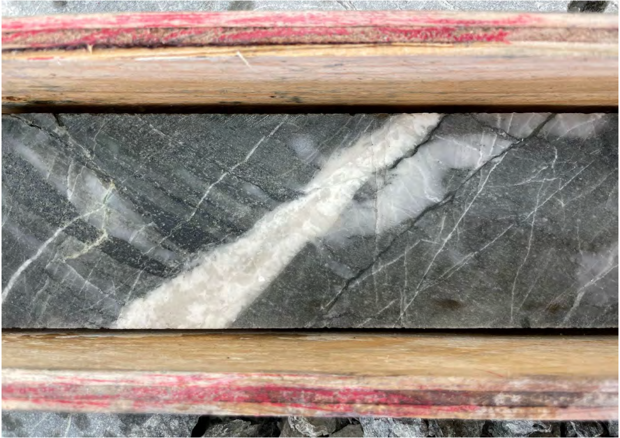
Cut HQ core sample of vein with quartz (translucent, off-white) and dolomite (opaque, bright white) with visible gold occurrence within vein. Mineral identification supported by SWIR spectral data (GS2337 @ 774.8m
