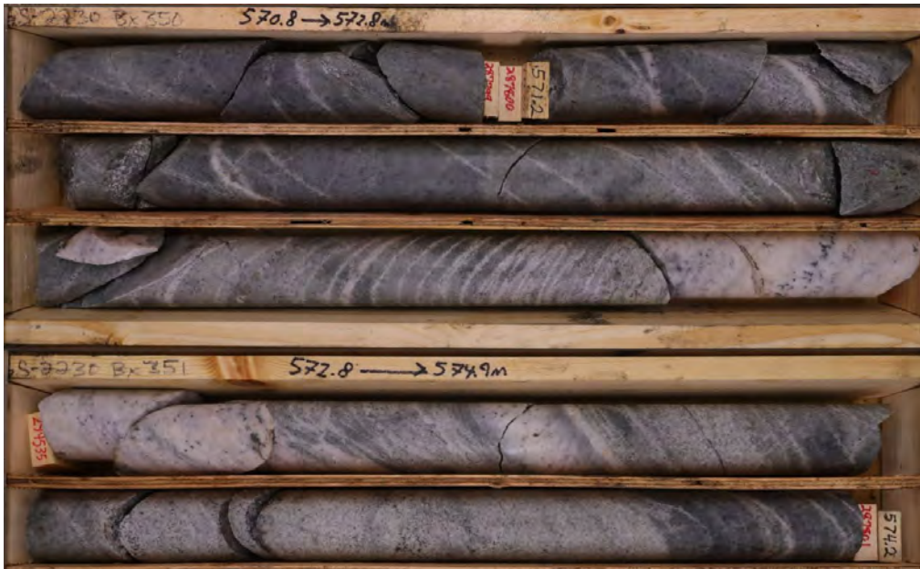
Figure 7-7 Stacked Quartz Veins cut by Visible Gold-bearing Sheeted Vein in Altered Tonalite
