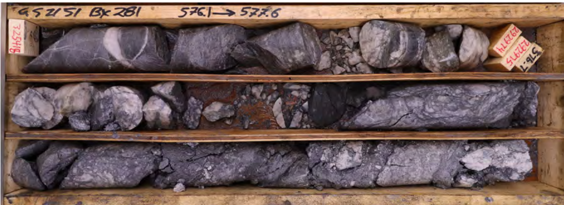
Figure 7-12 Breccia With Rehealed Matrix
