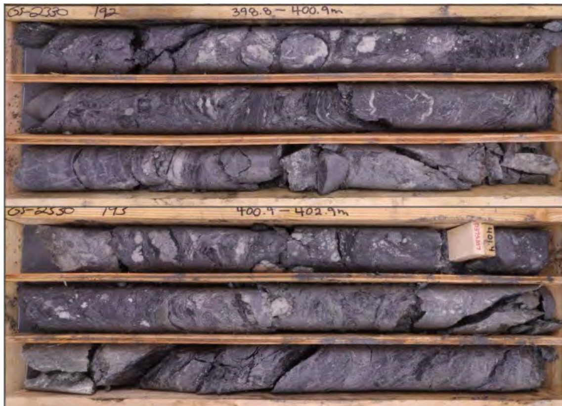
Figure 7-13 Cataclastic Breccia / Gouge With Rounded Quartz Vein Clasts
