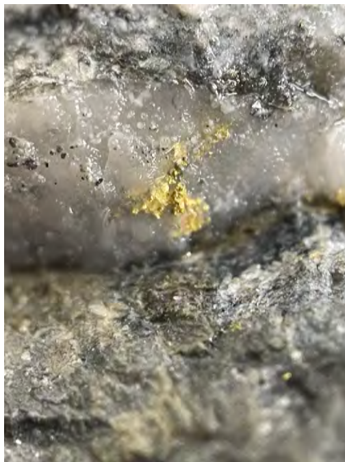
Figure 7-9 Gold in Quartz-Arsenopyrite Veinlet
