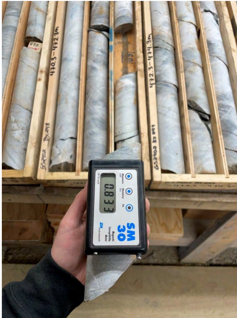
Figure 11-2 Magnetic Susceptibility Measurement
