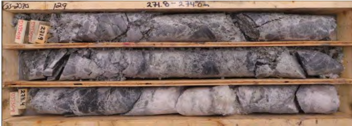
Figure 7-11 Breccia / Gouge With Rounded Clasts in Argillic Matrix
