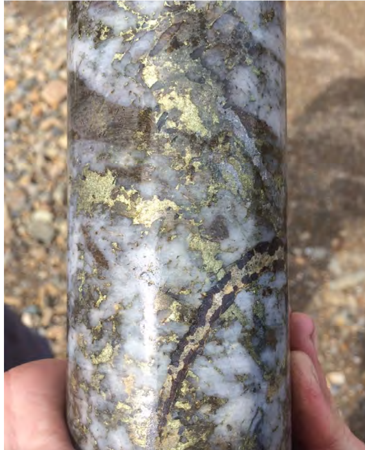
Chalcopyrite, wolframite and pyrrhotite in drill core
