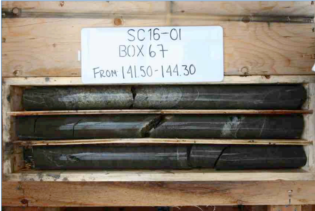
Figure 10.2.4 Core Photo From Hole SC16-01 0.605 ppm Au, 47.3 ppm Ag, Cu 1.99%, (141.6m – 144.6 m)
