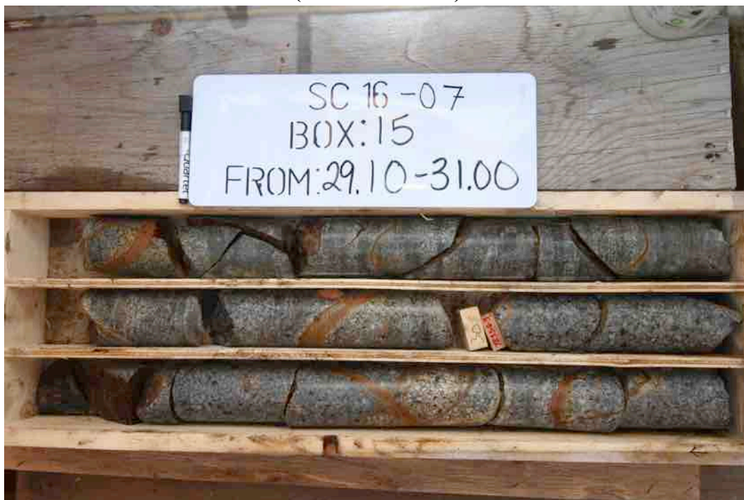
Figure 10.2.11 Core Photo From Hole SC16-07 0.011 Au, 1 g/t Ag, 2510 ppm Cu, 126 ppm Mo (27 m – 30m)
