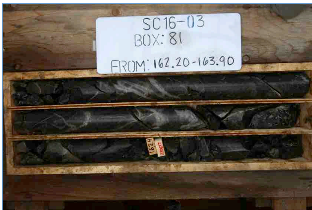
Figure 10.2.7 Core Photo From Hole SC16-03 747 ppm Mo, 380 ppm Cu, 1.1 g/t Ag (162.4 m – 164.7 m)
