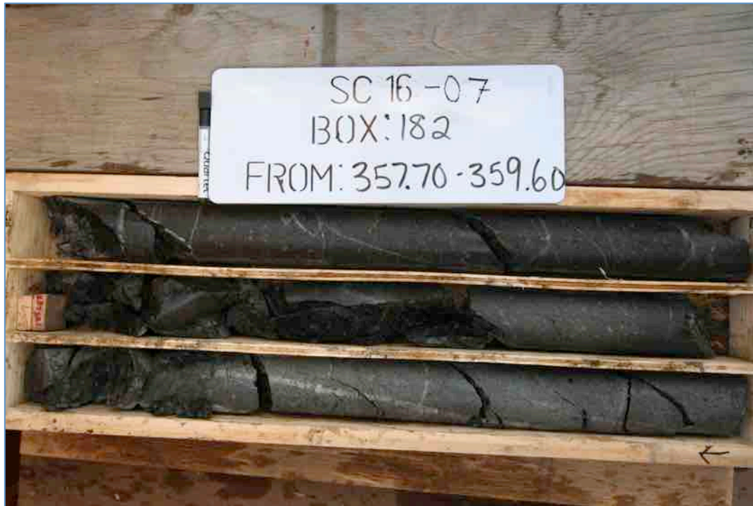
Figure 10.2.12 Core Photo From Hole SC16-07 2.8 g/t Ag, 0.016 Au, 1225 ppm Cu, 10 ppm Mo (357 m – 359 m)
