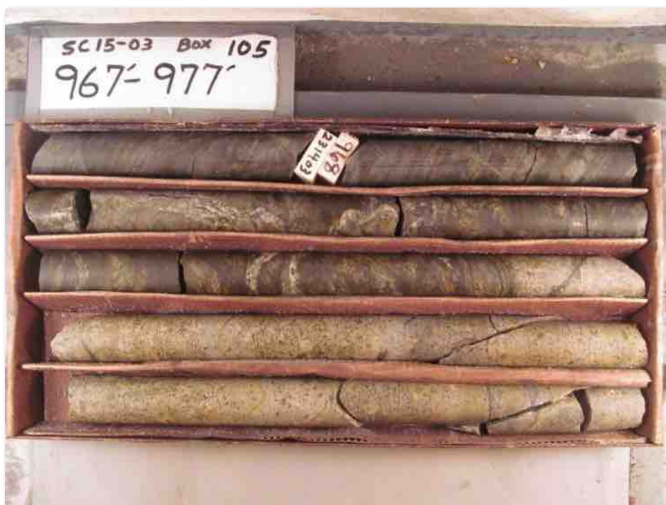
Figure 10.1.3 Core Photo From Hole SC 15-03 Assayed 0.29% Cu and 0.12 g/t Au
