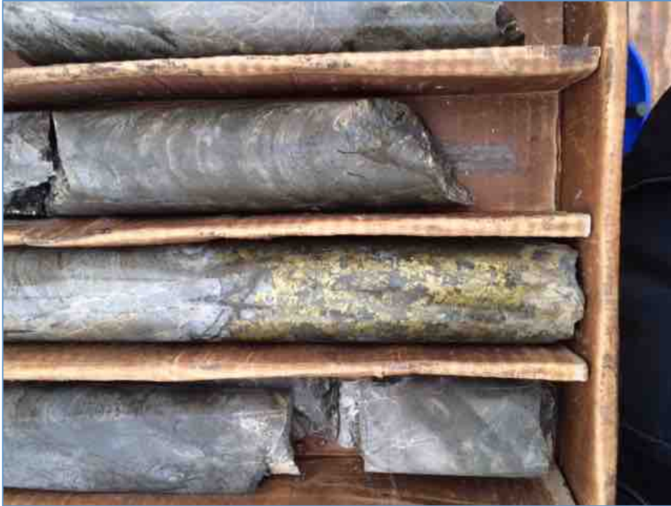
Figure 10.1.5 Core Photo From Hole SC15-03 Assayed 2.4% Cu and 0.46 g/t Au.
