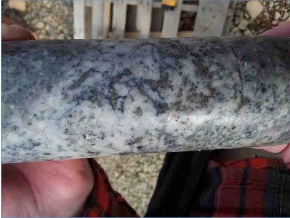
Figure 10.2.8 Visible Molybdenum Mineralization – Hill 1710
