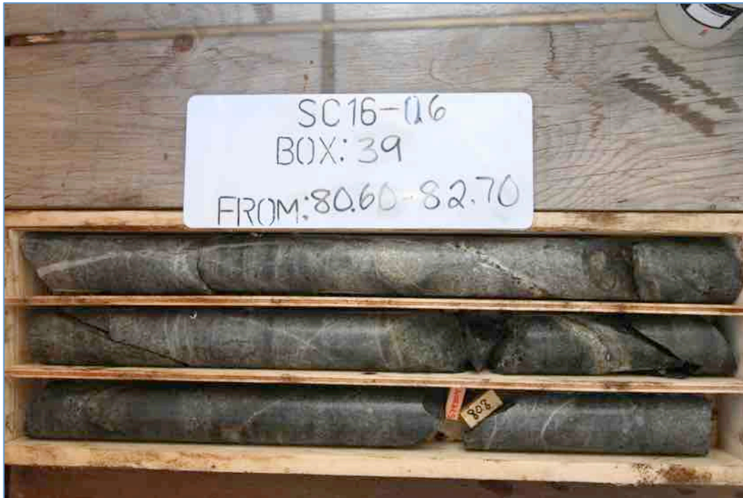
Figure 10.2.10 Core Photo From Hole SC16-06 0.013 ppm Au, 15.9 g/t Ag, 3730 ppm Cu, 282 ppm Mo (80.88 m – 83.9m)
