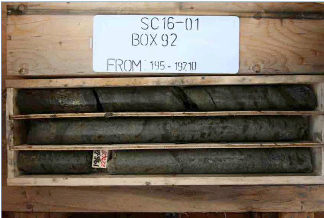
Figure 10.2.5 Core Photo From Hole SC16-01 0.112 ppm Au, 20 ppm Ag, Cu 1.07%, (196.5m – 198.6 m)
