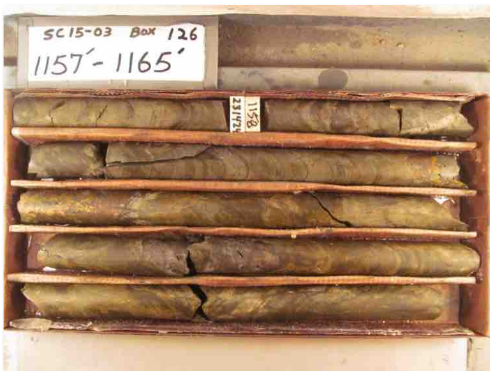
Figure 10.1.4 Core Photo From Hole SC15-03 Assayed 2.4% Cu and 0.46 g/t Au.
