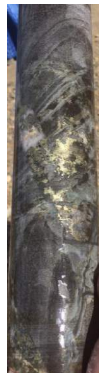
At least 3 phases of mineralization are present
