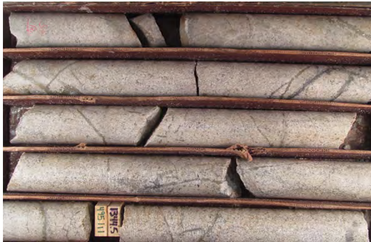
Argillic altered granodiorite with sulfide veins, 1.025 g/t
