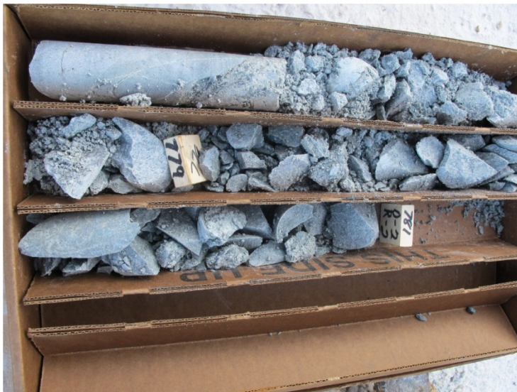
Figure 7.2.1B. Photo of drill core containing gold-bearing shear zone in the Dolphin stock.
