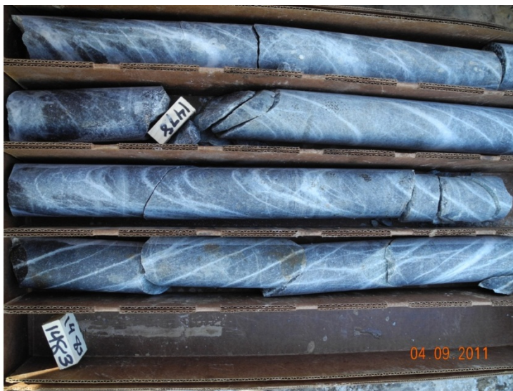
Figure 7.2.1A. Photo of drill core containing gold-bearing sulfide-quartz veinlets in the Dolphin stock.
