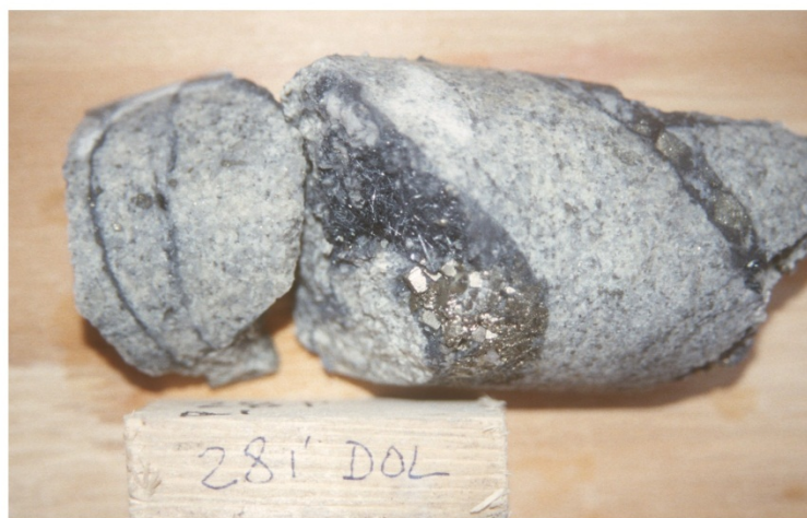
Figure 7.2.1C. Photo of drill core containing sulfide rich vein (pyrite-jamesonite) in the Dolphin stock.
